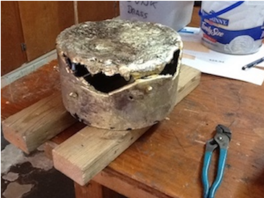
Failed Casting - not enough metal.
