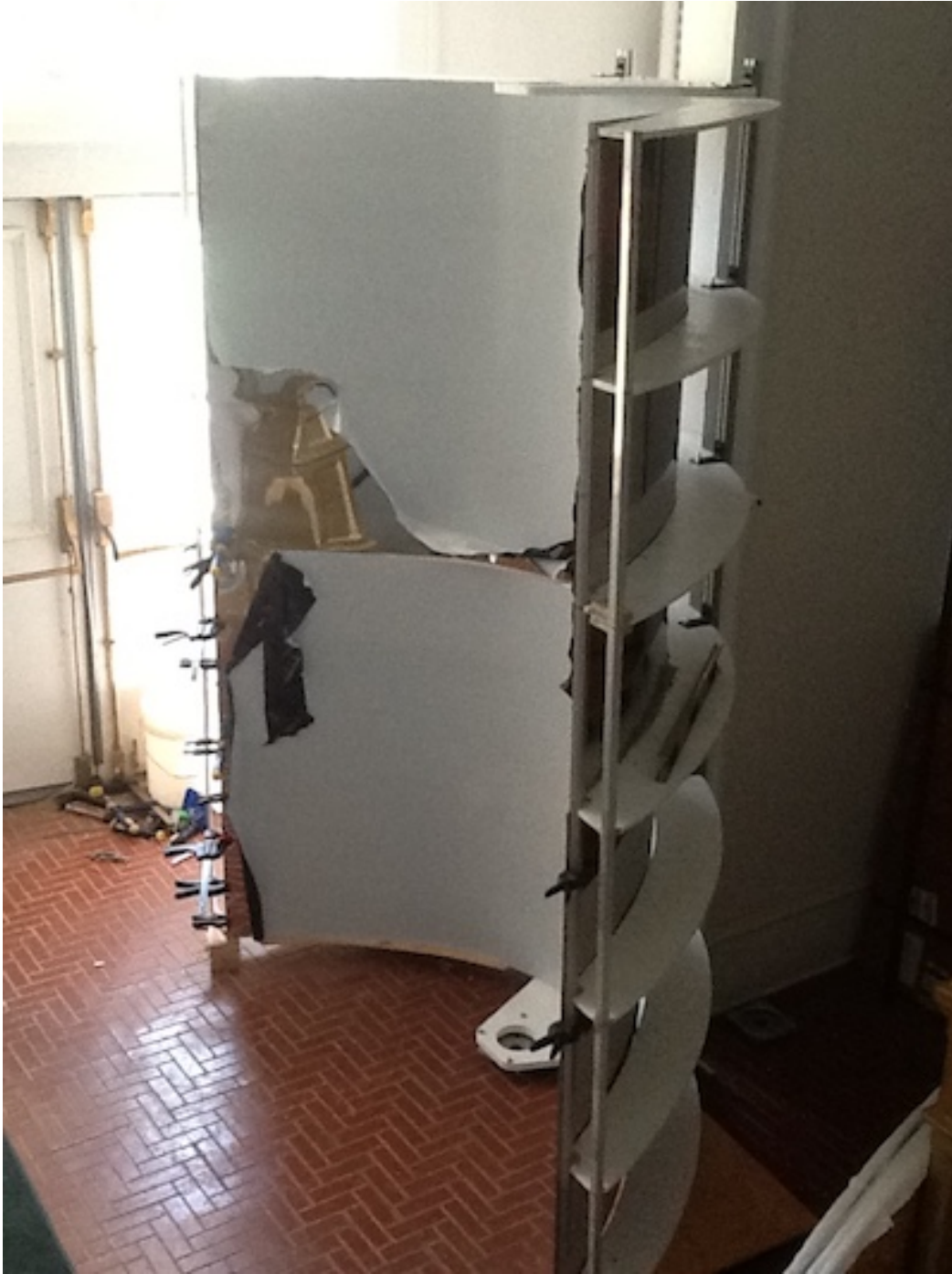
Solar Concentrator - second mirror install
